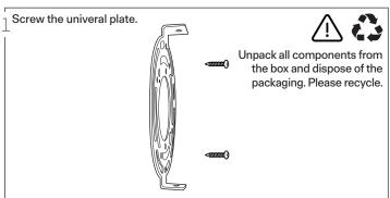
Use appropriate anchors and screws to fasten the universal plate for your installation.
