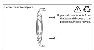
Use appropriate anchors and screws to fasten the universal plate for your installation.
