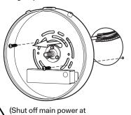
4 Adjust with level and secure by screwing
