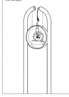
6 Carefully screw the disk in the center of the canopy. Place a hand under the disk to avoid any falls while installing.
