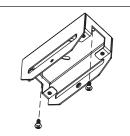
Pass sectioned flat cable in strain relief in canopy in direction of support box 3 and the other one in direction of support box 5. (Loosen captive screws for better passing of cable)
