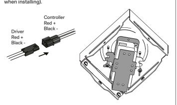
Screw support backplate on ceiling.(Screws not included)
