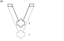
Pass sectioned flat cable in strain relief in canopy feed and canopy box. (Loosen captive screws for better passing of cable)
