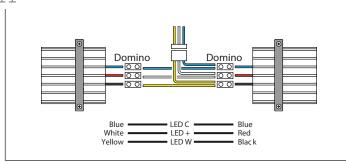
curving slightly the flat cable to pass the cover.
