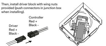
Fix non-feed canopy backplate on ceiling (screws not included).
