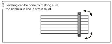
Repeat cable installation of steps 7 and 8 with support.
