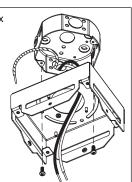
/ Make appropriate connextions with wire bundle provided to ceiling wiring. (Shut off main power at the circuit breaker panel)
