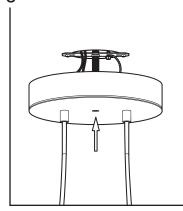
Screw the cap to the hollow stud to secure the canopy.
