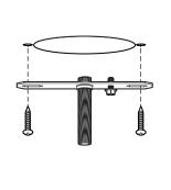
▲ First, connect the junction box ground to the green screw on the mounting plate.
