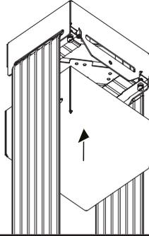
Then, screw in place with 2x flat screw provided. (Lift cable out of the way for better access)
