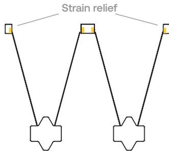
**7** Pass the flat cable in strain relief in canopy in direction of support box and screw it in place. (Loosen captive screws for better passing of cable)
