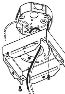
4 Make appropriate connexions with wire bundle provided to ceiling wiring. (Shut off main power at the circuit breaker panel)
