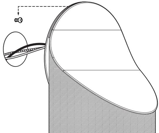
4 Once connected, mount the lamp on the wall by sliding the head of the screw in the aperture situated above the junction box.
