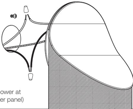
(Shut off main power at the circuit breaker panel)
